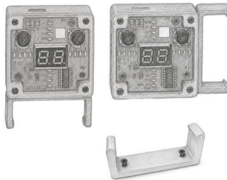
Illustration 2: Drillseye leg installation below or on the right side of the device
